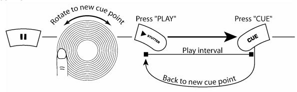
When the jog wheel is turned while paused, a new cue point can be located. By pressing "PLAY" while paused that point will be set. By pressing "PLAY" again (STUTTER) the point can be checked as desirable.
